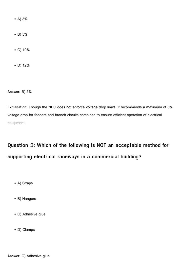
**Explanation:** The NEC requires mechanical support such as straps, hangers, or clamps for electrical raceways. Adhesive glue does not provide the necessary mechanical strength or reliability.
